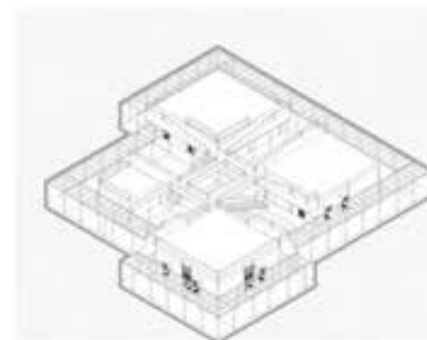
Diagram of the departmental module design, integrated with pergola walkways and rooftop terrace gardens, connected with open and semi-open spaces for practical classes, leading to an unconventional learning system.
