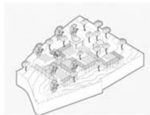
The design concept resulted in hierarchy of spaces, a sequence of open, semi-open and closed spaces connected with pergola walkways inducing nature in learning, hand in hand with preserving existing rich vegetation and features.
