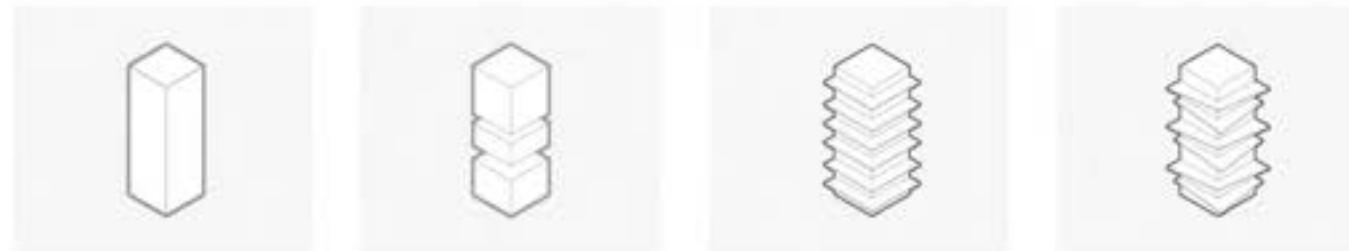
Analyzing the height of building through space requirement and structure study Demarcating the overall form with the area of usage - visitors & recreation - service and residential core Extruding cantilevers at each floor level from two faces to create a recreational yet provocative space Distorting the extruded cantilevers at different angles alternatively at every floor to create a dramatic space
