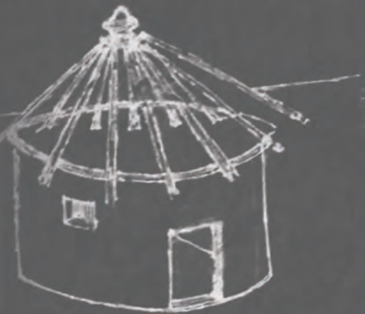
PLACING THE RAFTERS
