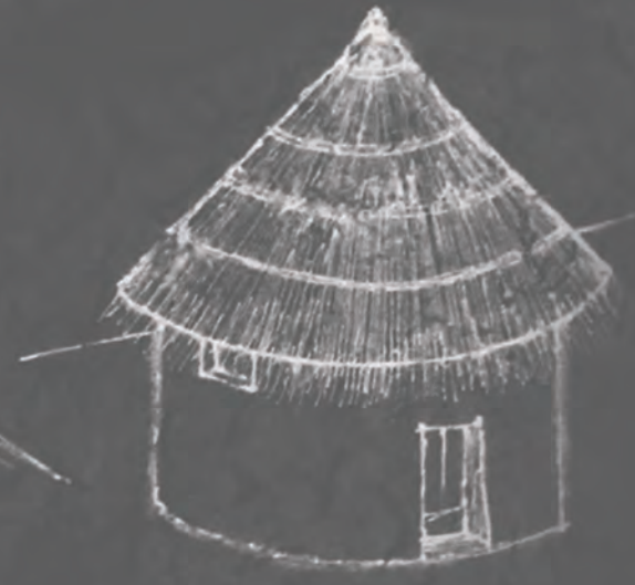
SECURING THE ROOF WITH ROPE
